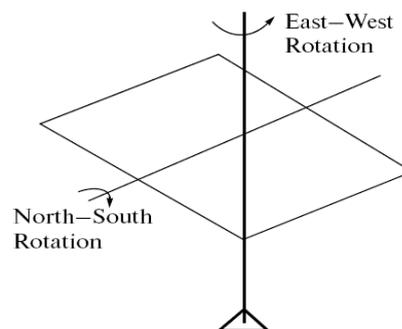
**Figure 3** – Dual axis tracking [8]
