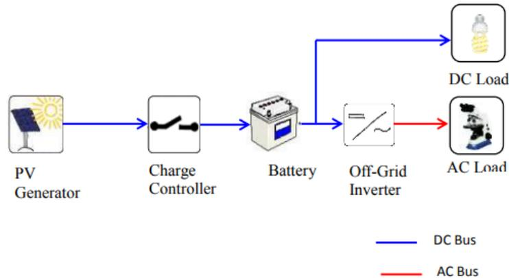
**Figure 1** – Shows principle of operation of solar PV system [7]
