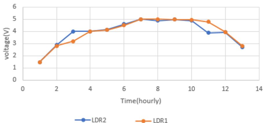
Figure 5 – Shows a one-day voltage profile of LDRs output for tracking system
