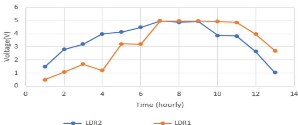
**Figure 4** – Shows a one-day voltage profile of LDRs output for fixed system
