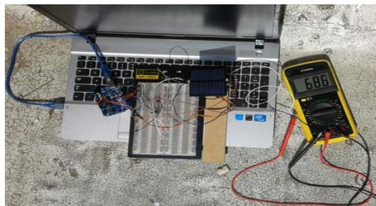
**Figure 3(b)** – Demonstration of tracking system with increased voltage output
