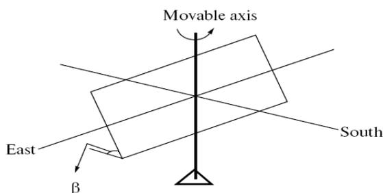
**Figure 2** – Single axis tracking [8]
